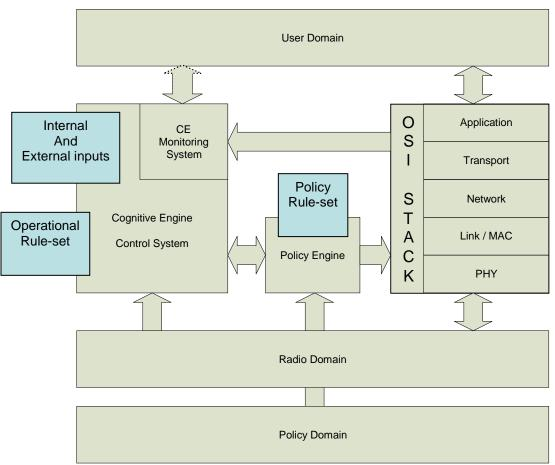
**Figure 1:** Conceptual view of Cognitive SDR Radio Architecture<sup>1</sup>
