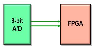
Serial connection (JESD204B) Pro Can handle high speed A/Ds
