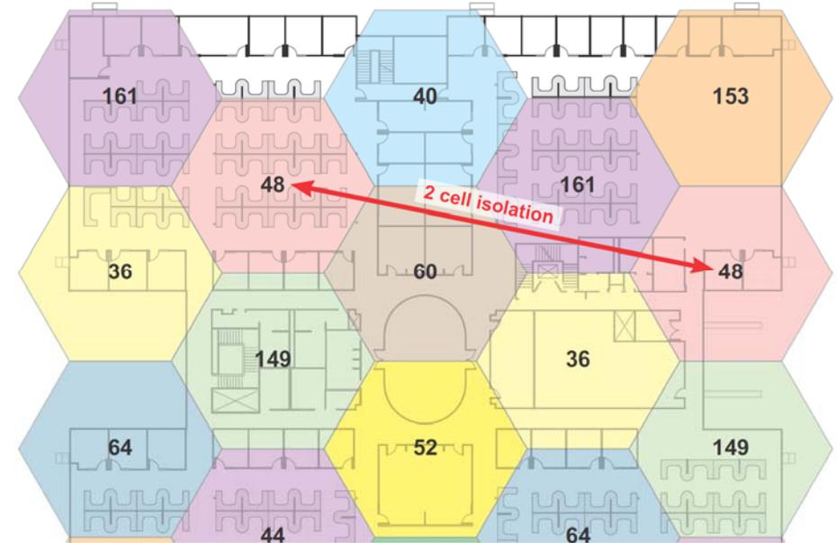
Wi-Fi uses combination of Energy Detect (ED) and/or Preamble Detect (PD) with Reuse={3-25} networks using C/N operation and consumer grade components
