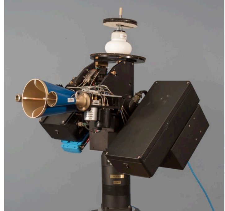
Tx and Rx equipment – mounted with antennas, pan/tilt units
