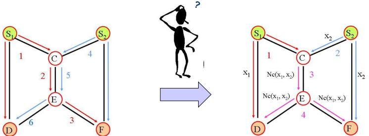
Protocol elements proposed to reroute the traffic to optimize the radio resources of a set of independant traffic flows.
