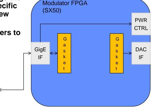
Gaskets reduce configuration management issues by not changing the platform specific and or waveform specific features during a porting effort.
