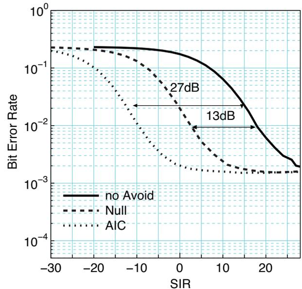
Fig. 4. The BER of WB-OFDM system vs SIR=10dB with AIC
