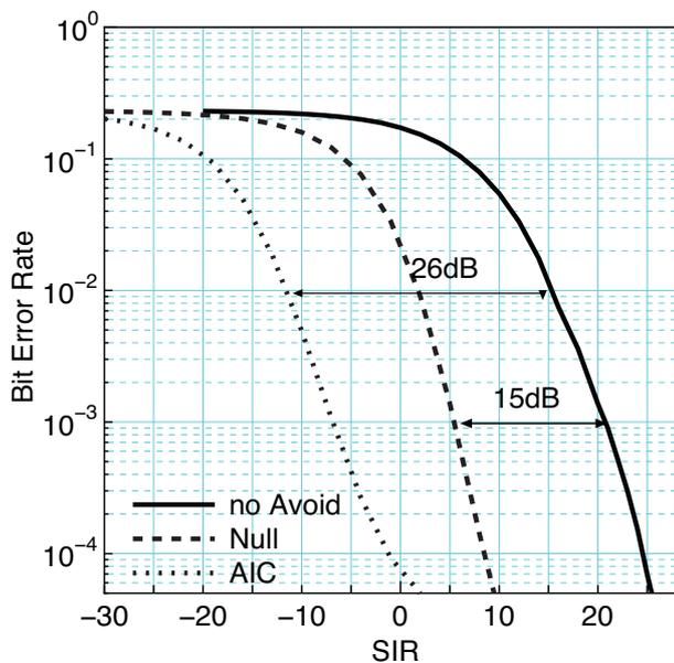
Fig. 5. The BER of WB-OFDM system vs SIR=15dB with AIC
