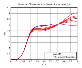
Figure 5. Extracted  $|NTF(e^{j\omega})|$  plot for all the  $f_s$ -modes when using opamps without constant-C scaling. Here, OSR = 16.
