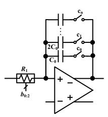
Figure 7. Schematic illustrating the resistor and capacitor bank selection for a single integrator.
