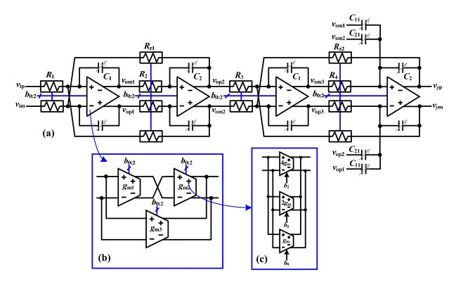
Figure 4. (a) Scalable CT- $\Delta\Sigma$  Loop-filter with constant-C scaling, (b) programmable two-stage opamps used in the loop-filter, (c) a digitally programmable transconductance element.
