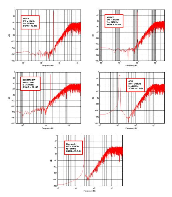
Figure 14. Simulated output spectrum of the reconfigurable CT- $\Delta\Sigma$  modulator for the modes: (a) WLAN ( $b_{2:0} = 011$ ,  $c_{2:0} = 001$ ), (b) WiMAX ( $b_{2:0} = 111$ ,  $c_{2:0} = 001$ ), (c) SDR with maximum bandwidth setting ( $b_{2:0} = 111$ ,  $c_{2:0} = 000$ ), (d) GSM ( $b_{2:0} = 000$ ,  $c_{2:0} = 101$ ), and (e) Bluetooth ( $b_{2:0} = 000$ ,  $c_{2:0} = 100$ ).
