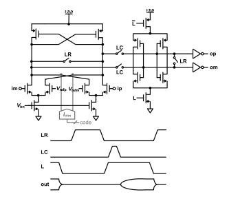
Figure 12. Comparator circuit used in the quantizer with timing diagrams[20].
