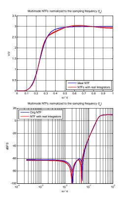
Figure 6. Extracted  $|NTF(e^{j\omega})|$  plots (linear and log y-axis) for all the  $f_s$ -modes with constant-C scaling of the loop-filter. Here, OSR = 16.
