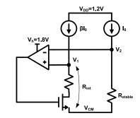
Figure 10. Schematic of the resistor tuning loop[18].
