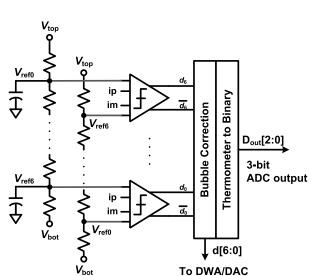
Figure 11. Schematic of the 3-bit Flash quantizer used in the ADC[19].
