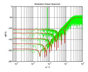
Figure 3. Fourth-order noise-shaping for each of the OSR modes shown in Table II. Here, the sampling frequency is normalized to 1 Hz and a 3-bit quantizer is used.
