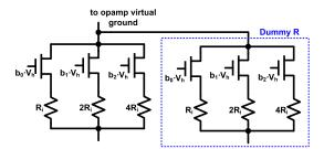
Figure 9. Programmable integrating resistors for  $f_s$ -scaling [18]
