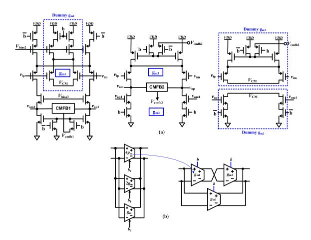
Figure 8. (a) A class-AB opamp cell used in the integrators. (b) 3-bit programmable class-AB opamp formed using the opamp cell.
