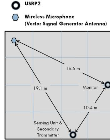
Fig. 3. Experimental Setup in the lab
