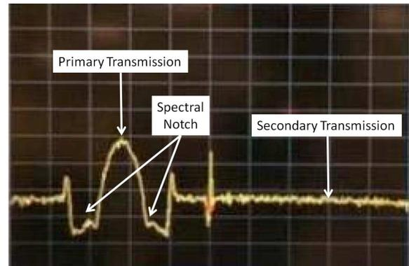
Fig. 6. Spectrum showing the co-existence of primary and secondary systems. [x-axis: 200 kHz/div, y-axis: 10 dBm/div]
