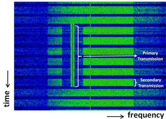
Fig. 2. Spectrogram illustrating the DSA operation
