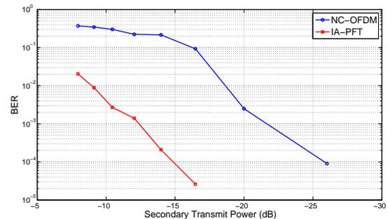
Fig. 7. BER at primary receiver vs. increasing secondary transmit power
