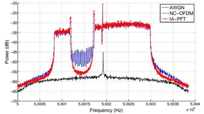
Fig. 5. RF transmitted signal spectrum of IA-PFT based NC-OFDM transmitter
