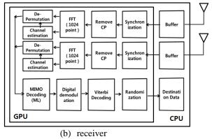
Figure 3. Block diagram of 2x2 SM MIMO WiMAX system
