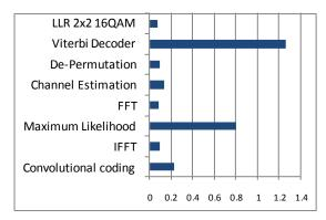
Figure 4. Computation time(ms) of 2x2 SM MIMO WiMAX system
