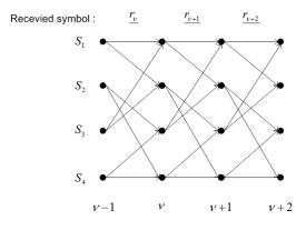
Figure 5. Trellis diagram of [2,1,3] Convolutional code
