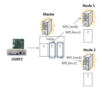
Figure 8. Inter-node data transmission using MPI
