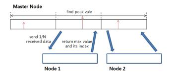
Figure 7. MPI-based Synchronization algorithm
