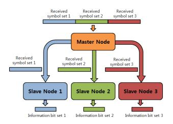
Figure 6. MPI-based Viterbi decoding
