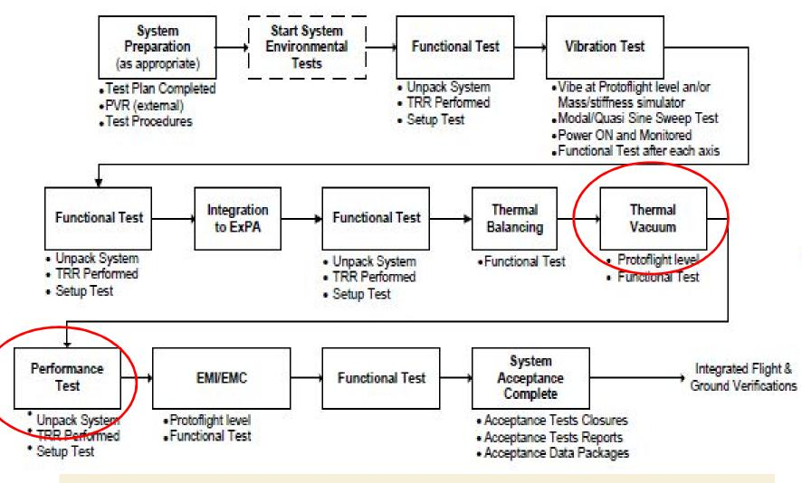
SDR Communications System Tests mixed among Environmental Tests
