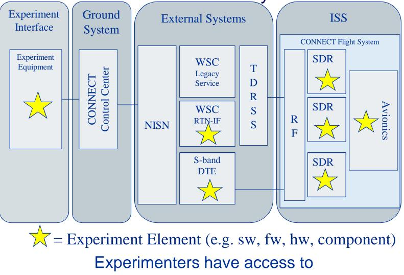
Flt SDRs, avionics, Gnd SDR, various ground points
