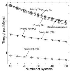
Fig.13 The throughput performance toward low priority channels while the average number of channel aggregation is 10.
