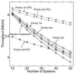
Fig.12 The throughput performance toward high priority channels while the average number of channel aggregation is 10.
