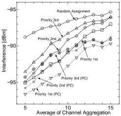
Fig.10 The given interference performance toward high priority channels while the number of systems is 10.
