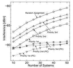
Fig.8 The given interference performance toward high priority channels while the average number of channel aggregation is 10.
