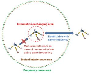
Fig1. Three areas for frequency assignment.
