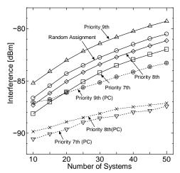
Fig.9 The given interference performance toward low priority channels while the average number of channel aggregation is 10.
