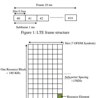
Figure 2: Resource Block structure of LTE
