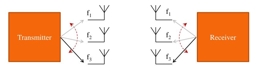
Instead of wideband antenna, a narrowband antenna with tunable frequency can be used, and hop between frequencies quickly
