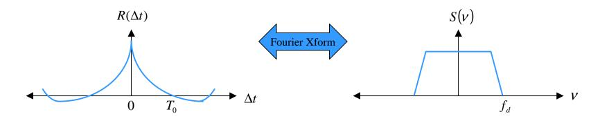
Time variations on the channel are evidenced as a Doppler broadening and perhaps, in addition as a Doppler shift of a spectral line.
