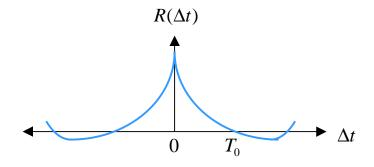
$R(\Delta t)$  specifies the extent to which there is correlation between the channel response to a sinusoid sent at time *t* and the response to a similar sinusoid at time *t*+ $\Delta t$ .
