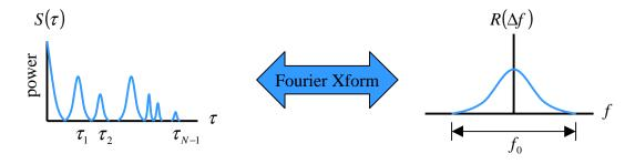
Compare coherence bandwidth  $f_0$  with transmitted signal bandwidth W:
