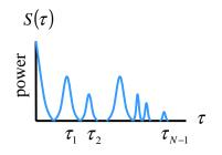
1. "maximum excess delay" or "multipath spread"  $T_m = \tau_{N-1}$
