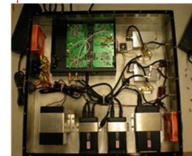
USRP in a casing with RF amps and power supply
