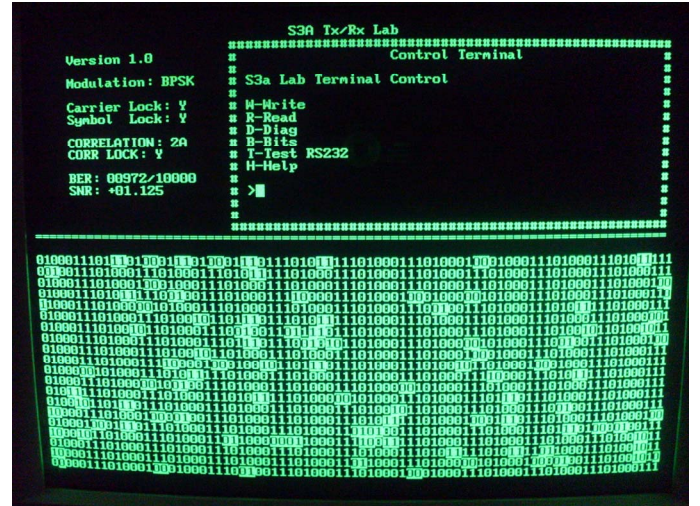
Fig. 3 – Screenshot of the control terminal with an SNR of 1.125 dB and the transmitted signal is the word 01000111. On the screen's top half we see on the left various receiver status metrics and on the right the control terminal. The screen's bottom part is a running display of the received bits, with erroneous bits denoted with inverse color. In this example, differentially encoded coherently demodulated BPSK is the modulation. Note that errors tend to occur in pairs of bits, which is expected due to the differential encoding and decoding [22 Sec. 4.2].
