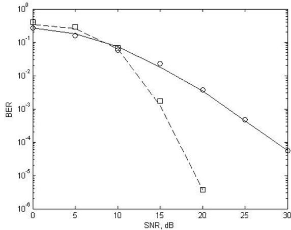
**Figure 7 Comparison of the simulated BER using the computer simulation vs the simulated BER using the test platform. 3km/h mobile speed. Uncoded BER and Coded BER, which are represented by the solid lines and dotted lines, respectively.**
