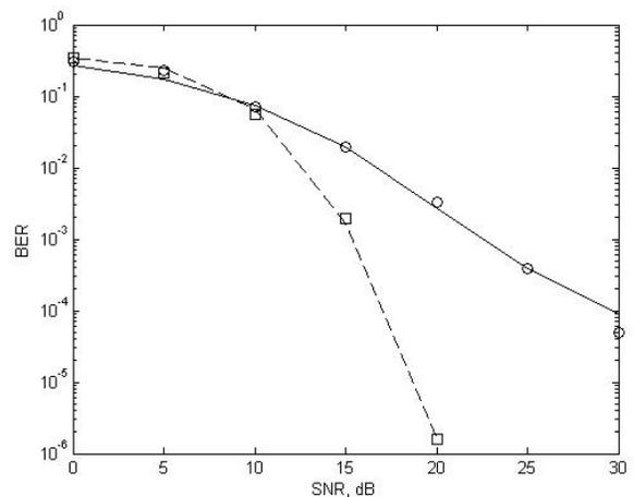
Figure 6 Comparison of the simulated BER using the computer simulation vs the simulated BER using the test platform. 60km/h mobile speed. Uncoded BER and Coded BER, which are represented by the solid lines and dotted lines, respectively.
