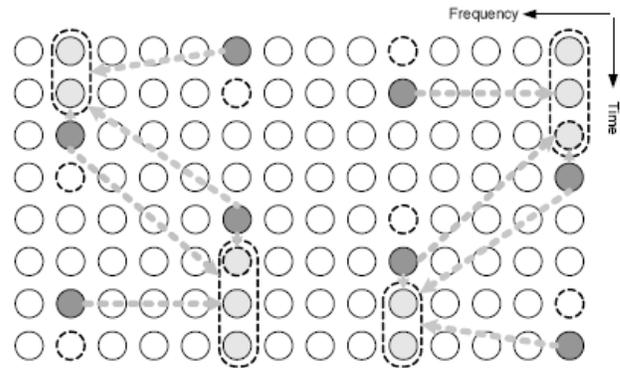
Figure 2 The advanced 2D interpolation channel estimation algorithm in 2 x 2 MIMO system
