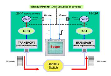
Figure 9: GPP-to-FPGA test facility
