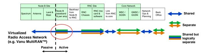
Figure 3. Infrastructure sharing possible with SDR. The red circle highlights the key change from traditional radios.
