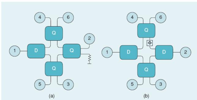
Figure 2: (a) SPI architecture using three hybrid couplers (Q) and one power divider (D). (b) SPI architecture using two power dividers (D), two hybrid couplers (Q), and a delay line.
