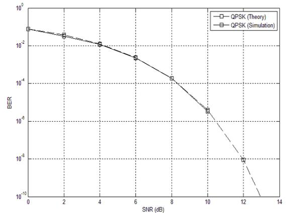
**Figure 8: BER simulation and theoretical results comparison for SPI test bench.**
