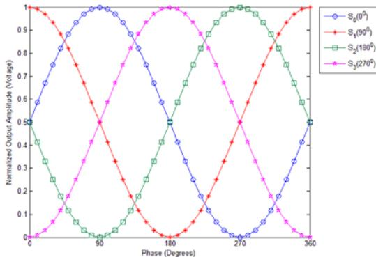
**Figure 6: SPI demodulator normalized output voltages versus phase difference between the input and reference signals at any frequency within the operating channel.**
