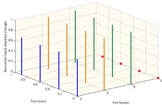
**Figure 7: Normalized output voltages at ports 3 to 6 of SPI demodulator for modulation state 2.**
