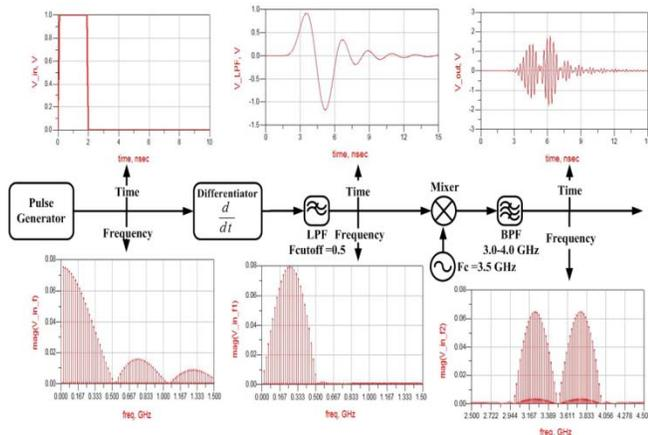
Figure 4: Block diagram for the generation of an UWB Monocycle pulse in 3.0-4.0GHz channel.
