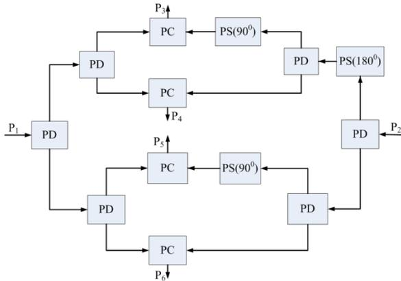
**Figure 5: SPI with the same architecture used as a modulator (note the arrow directions compared to Fig. 3).**
