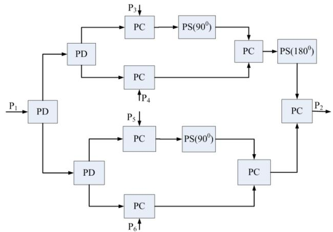
Figure 3: SPI architecture using power dividers/combiners (PDC) and phase shifters (PS).
