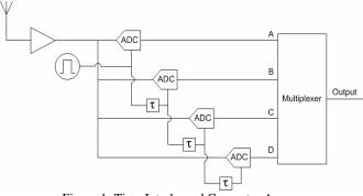
Figure 1: Time Interleaved Converter Array
