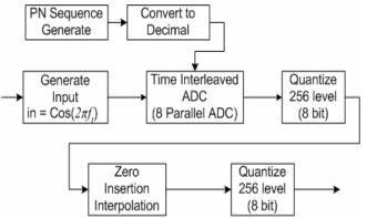
Figure 2: Block diagram of the interleaved ADC system
