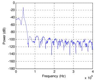
Figure 6: Power spectral density (PSD) of output of interpolator and RRC filter with pseudo-random jitter and skew (t\_adc) = 0.1 shows harmonics with significant improvement.
