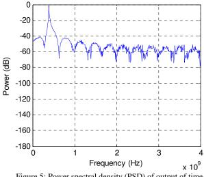
Figure 5: Power spectral density (PSD) of output of timeinterleaved ADC with pseudo-random jitter and skew (t\_adc) = 0.1 shows harmonics.
