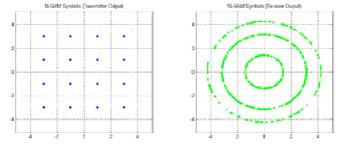
The received symbol constellation is spinning as predicted. And the phase rotation can be defined as:
