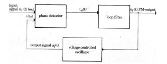
The loop filter is designed such that its DC output level is adjusted proportionately to the phase offset between the input sinusoid and the VCO output sinusoid. Assuming the feedback loop is stable, the input to the VCO will adjust the phase of the output sinusoid until its phase offset matches that of the input sinusoid.
