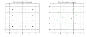
The constellation plots show the receiver QAM symbols are rotated by  $0.2\pi$  radians as predicted. Assuming that  $f_r \neq f_t$  and that  $(f_r - f_t) = 10$ Hz then the received baseband symbol stream can be defined as:
