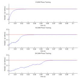
In addition, the plots below show that the algorithm successfully tracks a varying relative carrier phase at the receiver:
