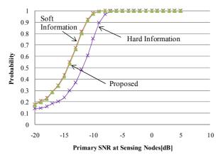
Fig. 7. Detection  $P_D$  of the proposed cooperative sensing. Subcarrier detection threshold is 11.5[dB].
