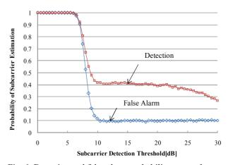
Fig. 6. Detection and false alarm probability versus the subcarrier detection threshold.Primary SNR of each sensing node is -15[dB].
