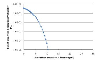
Fig. 4. False subcarrier estimation probability versus the subcarrier detection threshold at the master node. Primary SNR of each sensing node is -15[dB].
