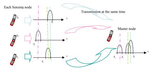
Fig. 3. Image of proposed information exchange method by using OFDM signal structure.
