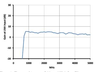
Figure 4: Flatness of Antenna, Cable, and High-Pass Filter
