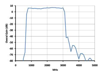
Figure 7: Data Collection Gain with Post Processing
