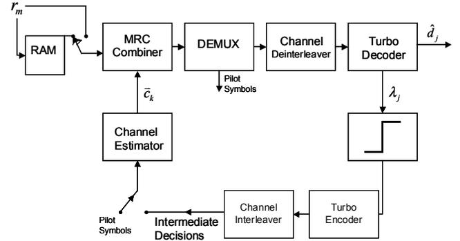
Figure 2 Turbo-Aided Receiver Model
