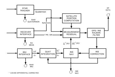
Figure 7 NAVSYS GPS/Inertial Filter Software
