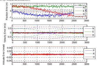
Figure 8 Attitude, Position, and Velocity Estimation Error without Star Tracker Updates
