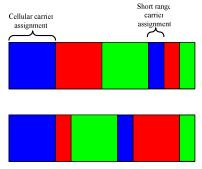
Figure 6 Example of non-contiguous carrier assignment
