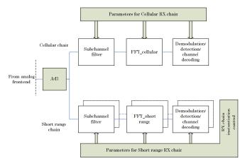
Figure 7 SDR receiver concept
