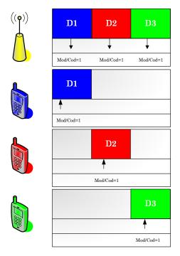
Figure 5 Carrier allocation scenario with no cooperation and static carrier assignment
