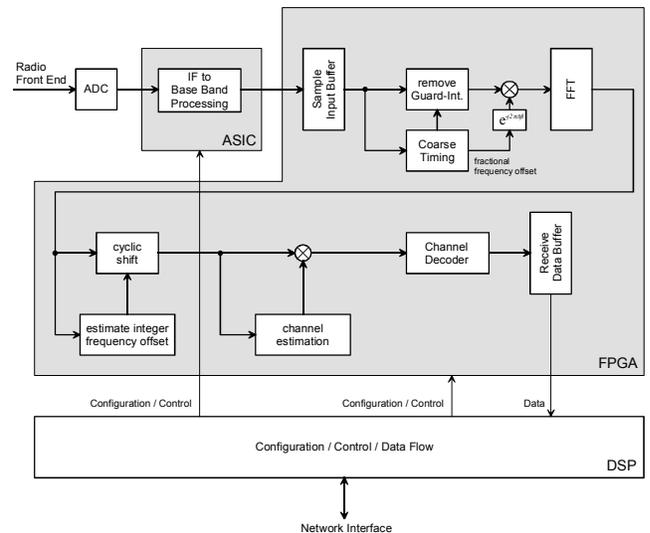
**Figure 7: Receiver structure including which processing element performs which tasks.**
