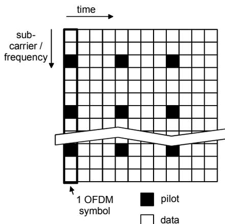
**Figure 3: Placement of pilot symbols used for channel estimation in an OFDM transmission.**
