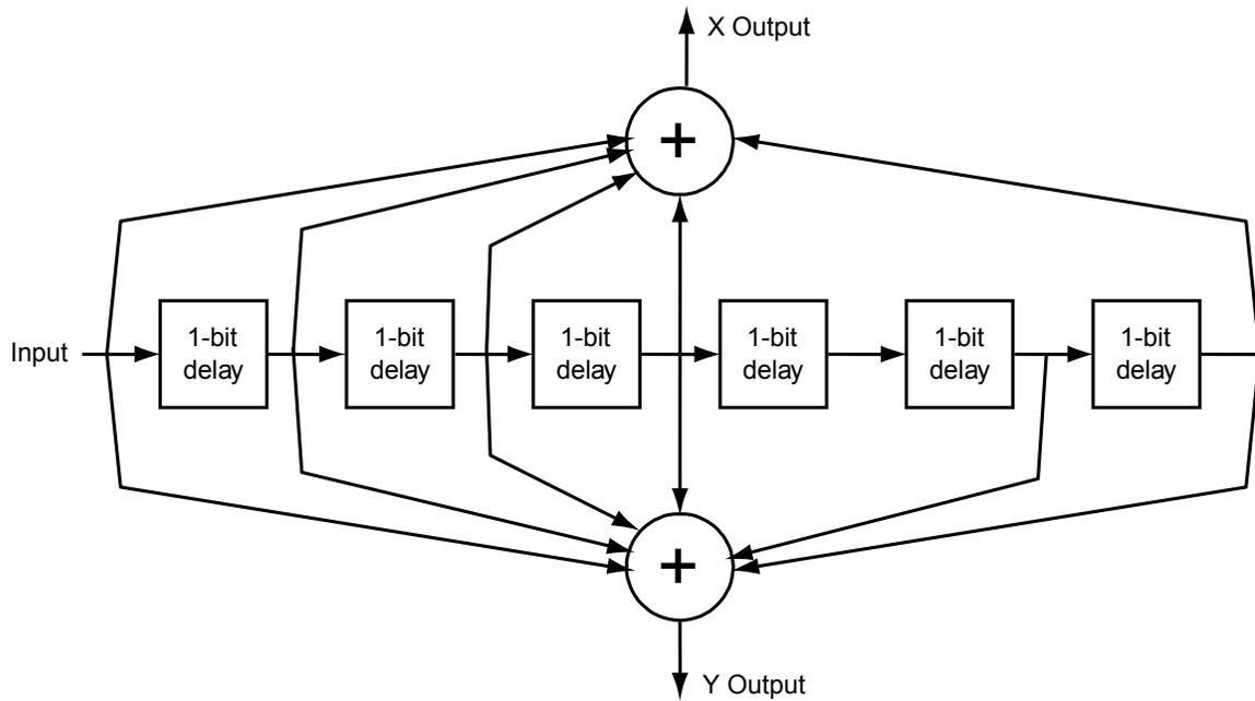
Figure 3 Convolutional Encoding with Constraint Length of 7 and  $\frac{1}{2}$  Rate
