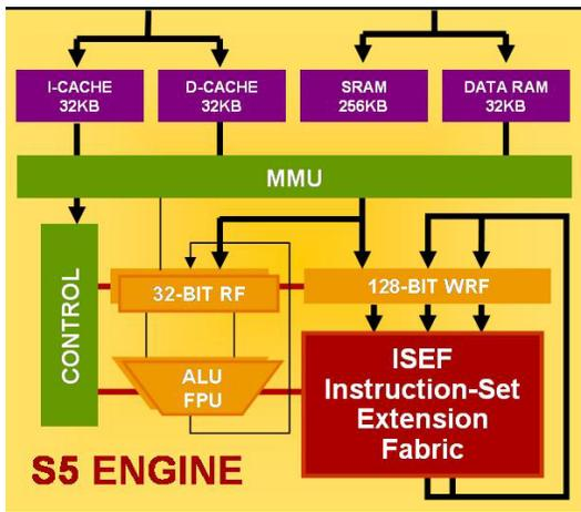
Figure 2 Software-Configurable Processor Architecture
