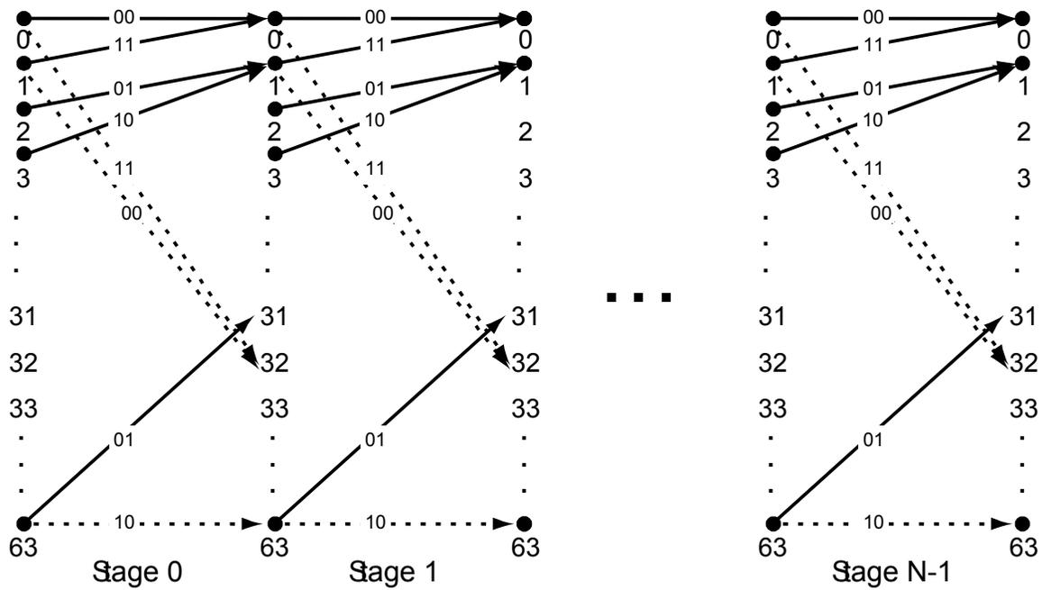
Figure 4 Trellis Diagram for  $\frac{1}{2}$  Rate and Constraint Length of 7
