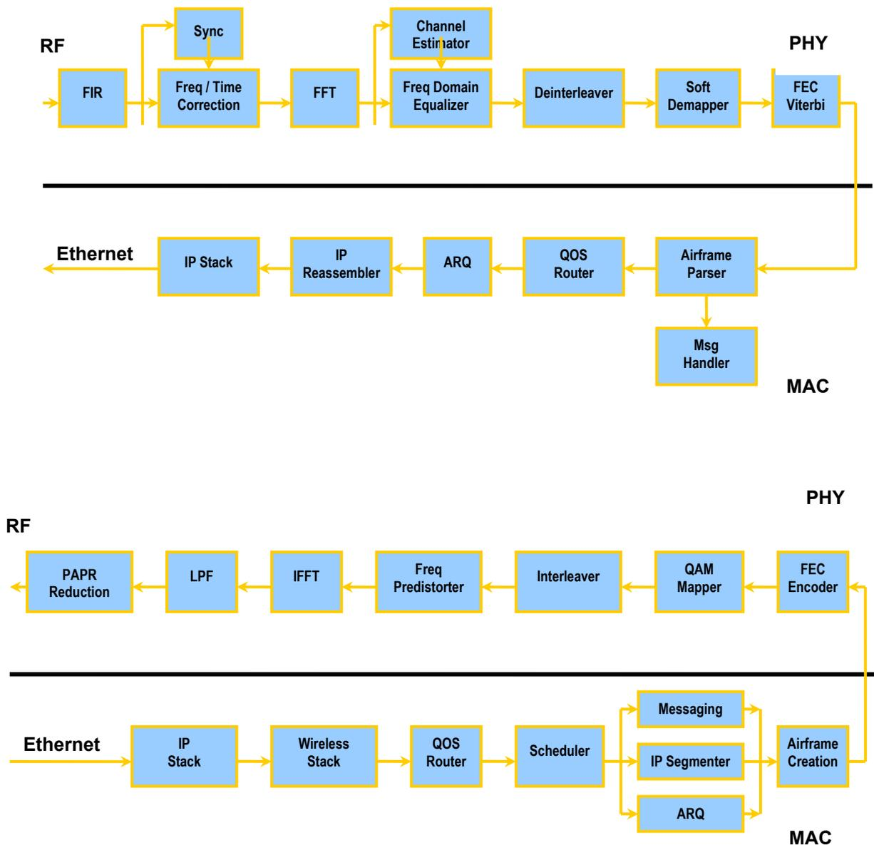
Figure 1 802.16 Receiver and Transmitter
