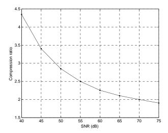
Figure 4: A signal's rate-distortion curve provides SignalZIP and Samplify users with a one-click summary of the range of tradeoffs between bit rate and signal quality available from compression.
