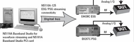
The Baseband Studio for waveform streaming solution can achieve data rates up to 40 MSa/s. This translates into 20 MHz of bandwidth for each of the I and Q channels and a total RF modulation bandwidth of 40 MHz. This wide bandwidth enables simulation of multiple channels of communication signals or generation of pulsed waveforms. The data rate is continuously displayed on the software graphical user interface (GUI) and is available on the API.
