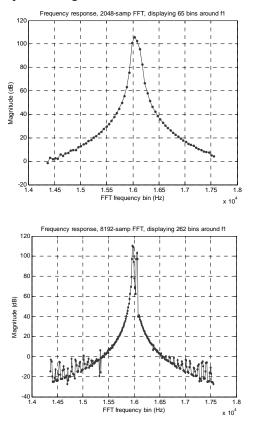
Figure 1: Compressing snapshot RAM captures improves FFT resolution from 25 kHz/bin (4k FFT; top) to 6.25 kHz/bin (16k FFT, bottom), allowing closely spaced signals to be resolved.
