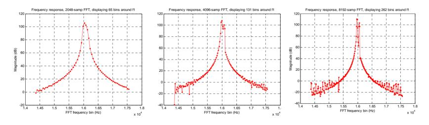
N = 4096 before Samplify FFT resolution: 100M / 4k = 25 kHz N = 8192 Samplify @ 2:1 FFT resolution: 100M / 8k = 12.5 kHz N = 16384 Samplify @ 4:1 FFT resolution: 100M / 16k = 6.25 kHz
