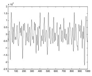
Figure 2: A two-carrier 3G wireless waveform with ACLR of 85 dB can be compressed by 2:1 (ACLR = 77 dB) or 3:1 (ACLR = 61 dB), thus improving both snapshot RAM-based and disk drive-based arbitrary waveform generators.
