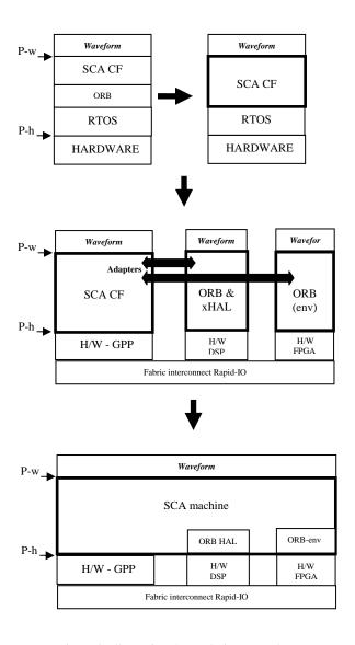
Figure 3: Illustrating the evolutionary path to an SCA machine
