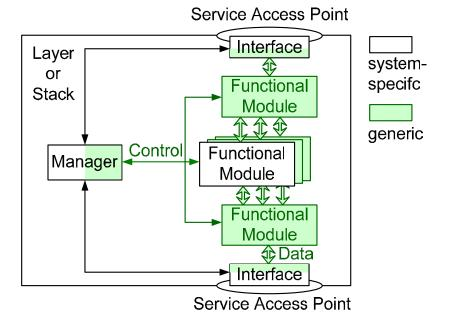
→ Simulation and performance evaluation on several levels: (sub-)layer as well as complete protocol stack
