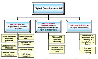
novel features of digital The this spectrometer are enabled by broadband, highfidelity digitization and ultrafast (20-40 Gbps) digital processing of RF waveforms, using superconductor rapid single flux quantum (RSFQ) technology. Two central elements of such a digital-RF receiver, the ADC and the digital correlator, have already been demonstrated by HYPRES in the laboratory. The low noise, high linearity, and high dynamic range of the superconductor ADC permits high-fidelity
