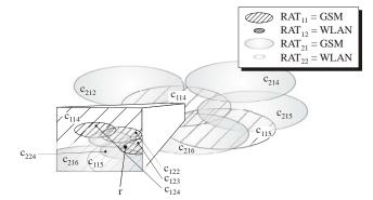
Figure 3: Area covered by GSM and WLAN cells cijk of Network Providers, NP<sub>1</sub> and NP<sub>2</sub>
