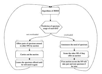
Figure 5: Mechanism of dynamical spectrum pooling in DNMP for cell c<sub>iik</sub> of RAT<sub>ii</sub> of NP<sub>i</sub>
