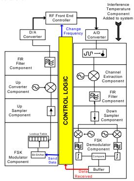
Figure 3: FSK Software Radio with Interference Temperature Component
