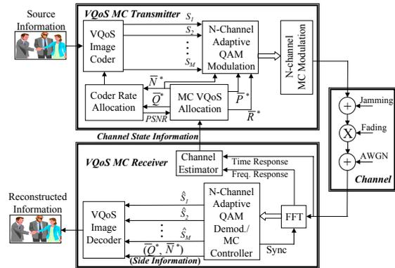
Figure 1: Joint VQoS MC image coding system.
