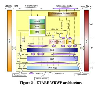
The Convergence Sublayer (<u>CS</u>) carries out the interface with different types of services and manages the sessions (IP, connection-oriented, connectionless short messages, etc.). It makes use of Ad Hoc Mobility Management (AHMM) services to access a coverage area.
