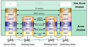
Figure 4 – Example of regenerative relaying Peer to peer User Plane protocol end points
