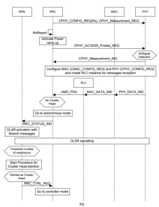
Figure 3 – Example of simplified inter-layer messages exchanges for transitions from flat network to clustering and hierarchical organisation together with routing
