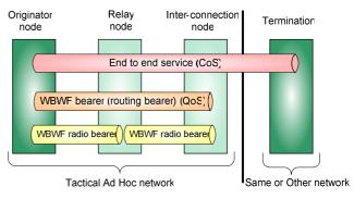
Figure 1 – ETARE WBWF QoS Architecture
