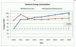
Figure 5 – An overview of how the energy consumption develops for the two cases. This graph is represents the case with an aggressive traffic growth.
