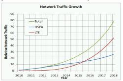
Figure 2 – Predicted traffic growth at an average rate of 70% per annum, representing the aggressive traffic growth rate. The figure also shows how the traffic is divided between the two network layers.
