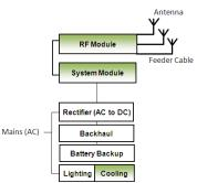
Figure 1 – Modular overview of some of the main components in a typical macro base station.
