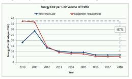
Figure 6 – How the energy efficiency of the network evolves. In the reference case, the first year is optimistic since it assumes more efficient equipment.
