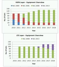
Figure 4 – A comparison to show which equipment is used for the different layers of the network. It is possible to note that most of the replacement is carried on the HSPA layer (early years), removing less efficient equipment.
