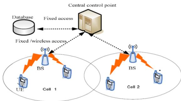
Figure 1: Database driven access to TVWS
