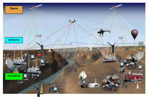
Figure 1: The Three Layers of Recovery Communications
