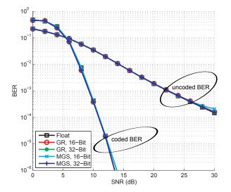
Fig. 8. Coded and uncoded BER for MGS and GR-plain implementations with 16-Bit and 32-Bit I/O data-width
