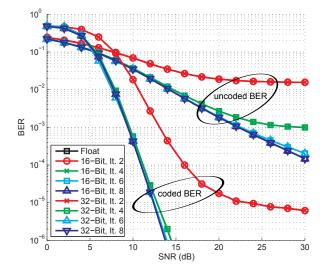
Fig. 9. Coded and uncoded BER for CORDIC based implementations with 16-Bit and 32-Bit I/O data-width for different CORDIC iterations
