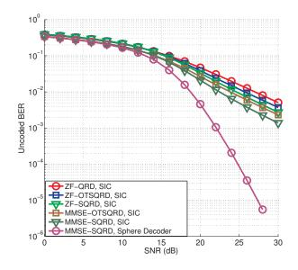
Fig. 1. Uncoded BER performance of a  $4 \times 4$  MIMO system using 16QAM modulation for different MIMO preprocessing schemes
