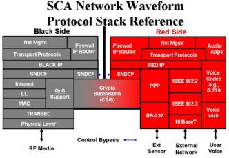
Figure 11. Networking waveform protocol stack reference model developed by SDR Forum Waveform Component Study Group. (Source: SDR Forum [10]). Application (Awareness,
