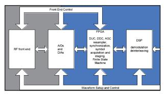
Figure 5. Black side control and data flow architecture. (Source: Maier, Spectrum Signal Processing)
