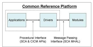
Figure 10. Common Reference Platform procedural and message passing interfaces between applications, drivers and modules.
