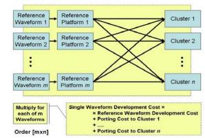
Figure 2. Waveform "porting" costs without a Common Reference Platform can grow by order [m X n].
