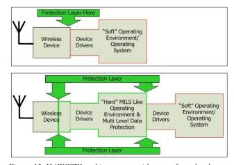
Figure 13. HAWCS<sup>™</sup> architecture provides waveform developers with an approach for securing the SDR platform from wireless and network "hacking".
