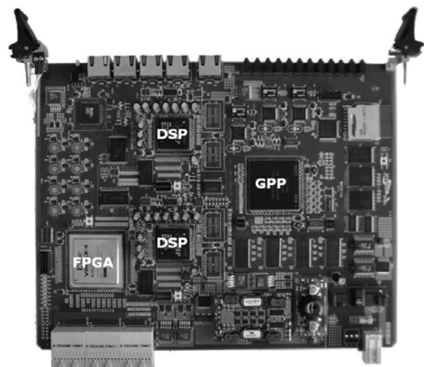
Figure 6: Photograph of implemented Baseband Signal Processing part of SDR smart antenna system.
