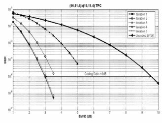
Fig. 3. BER vs.  $E_b\!/N_0$  of product code [BCH  $(16,\!11,\!4)^2]$  on a Gaussian Channel
