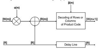
Fig.1. Block diagram of elementary TPC decoder (m<sup>th</sup> half-iteration)
