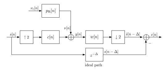
Fig. 5. System set-up for study of a half symbol-spaced equalizer.
