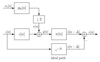
Fig. 4. System set-up for study of a symbol-spaced equalizer.
