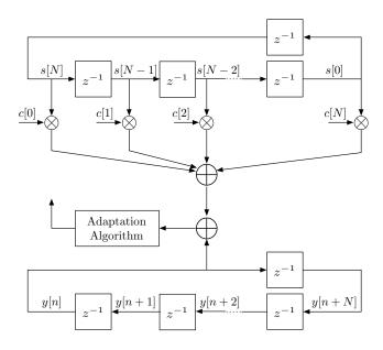
Fig. 7. The system set-up for a symbol-spaced cyclic channel identification.
