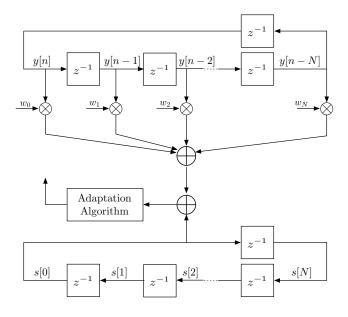
Fig. 6. The adaptation set-up for a symbol-spaced cyclic equalizer.
