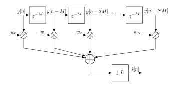
Fig. 3. Details of a fractinally-spaced equalizer with tap-spacing  $(M/L)T_b$ .
