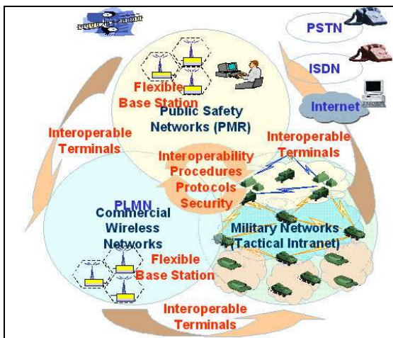
Figure 7: SDR based System Architecture for Interoperability
