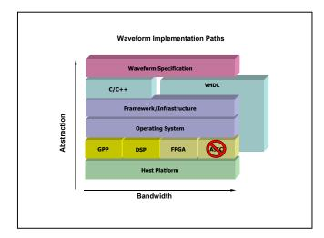
Figure 1: Software Radio Abstraction Layers
