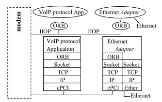
Figure 6. VoIP Application Block Diagram
