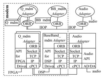
Figure 5. Voice Application Block Diagram
