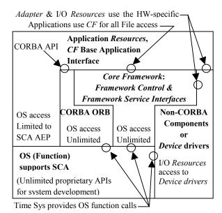
Figure 4. Relationship between OE and Application (No *Devise Interface* is provided)
