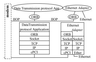
Figure 7. Data Transmission Application Block Diagram
