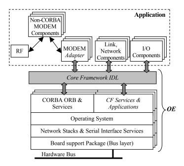
Figure 3. Software Structure
