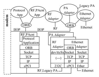
Figure 8. RF/PA Utility Application Block Diagram
