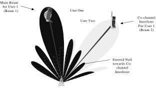
Figure 3 – Adaptive Array Principles
