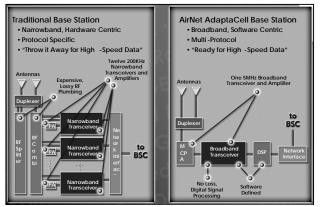
Figure 1 – AdaptaCell BTS Architecture
