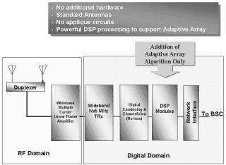
**Figure 2 – Software Upgrade for Adaptive Array**
